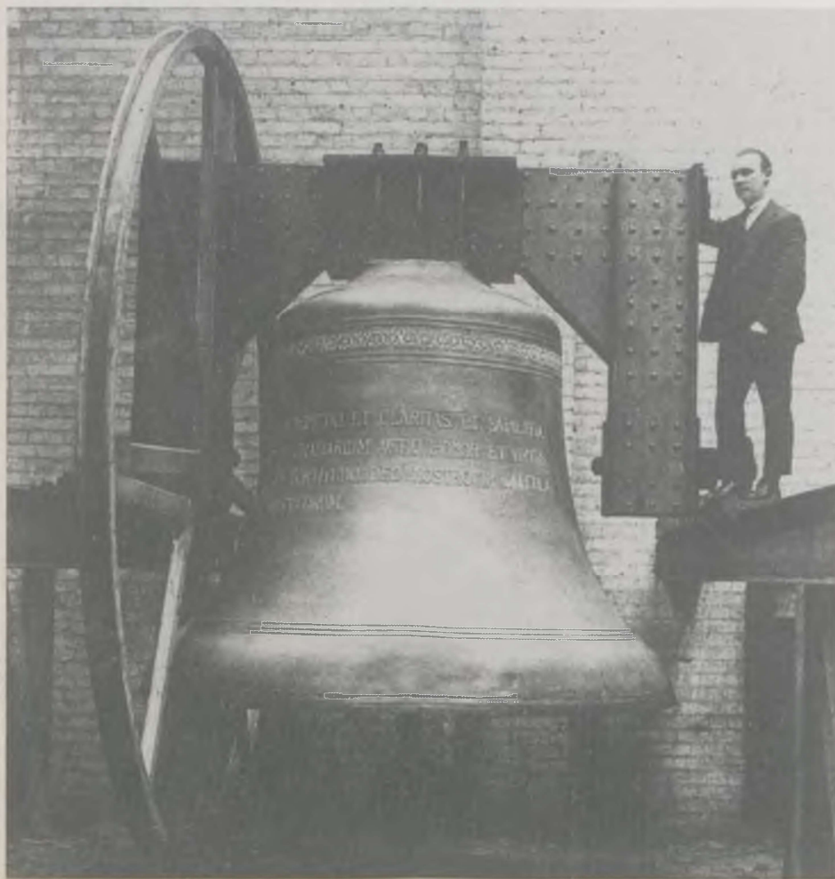
A special frame was erected in Taylor's works for testing the bell – Pryce Taylor is on guard!
